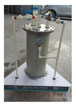
**PIPES AND FITTINGS**- Use of only National Safety Foundation (NSF, USA) certified CPVC pro pipes, valves, fittings and unions manufactured by ASTRA India, Ahmedabad, Gujarat. Guaranteed life 30 years. Non-corrosive and not affected by chlorine solution at all.
